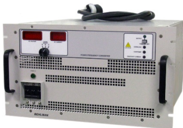
Behlman FC5003 is a “turn-key,” rugged COTS frequency converter that converts 120/208 VAC, 3-phase, 60 Hz ground power to 115/200 VAC, 3-phase, 400 Hz aircraft power at 6000 VA, 16 Amps per phase.
