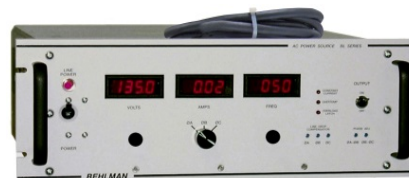
Behlman BXL3X500 is a “turn-key,” rugged COTS frequency converter that converts 115 or 230 VAC, single-phase, 47/63 Hz power to 115/200 VAC, 3-phase, 400 Hz at 1500 VA, 4.3 Amps per phase.
