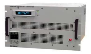
There's also a unique overload protection system that folds back voltage to maintain rated current without output waveform distortion. Units are supplied with RS-232 remote control and 28 VDC control of Output On/Off. In addition the unit has provisions for slide mounting.
